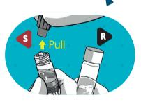
Pull the cap off the solvent syringe.
